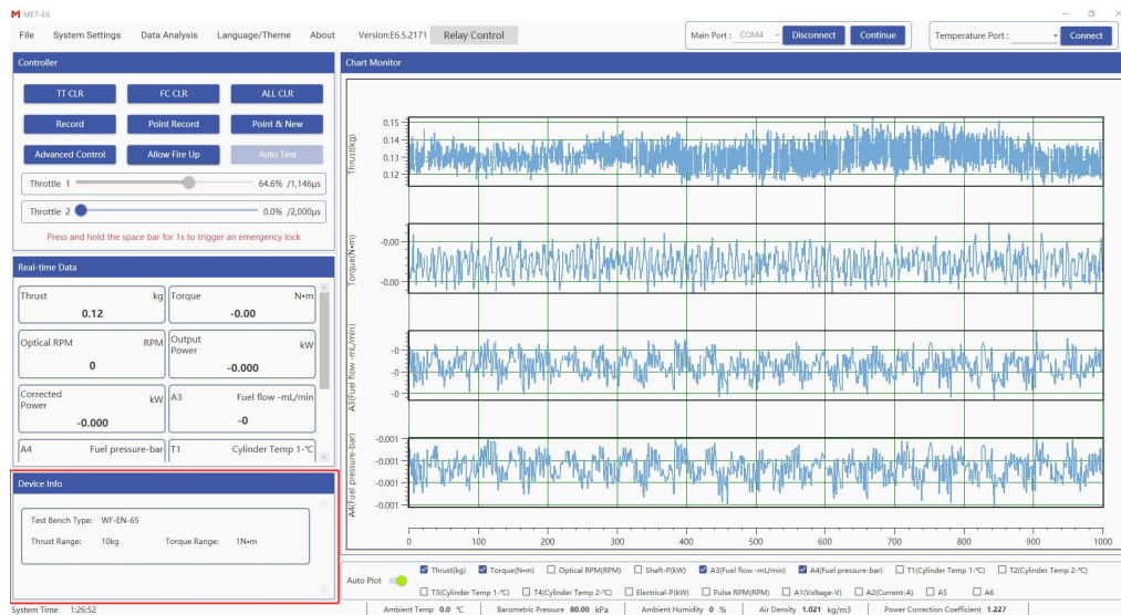
Figure 5-4-1 Device information window interface
