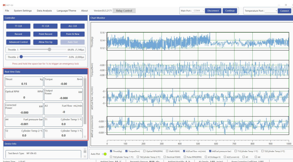
FIG 5-3-1 Real-time data window interface
