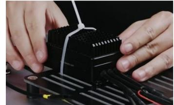
FIG 4-2-1 ESC installation and commutation speed line connection
