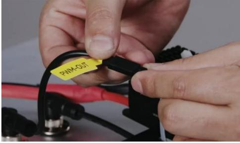
FIG 4-2-3 Signal line to PWM out
