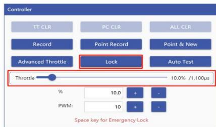
FIG 4-5-1 Unlock the throttle and drag it
