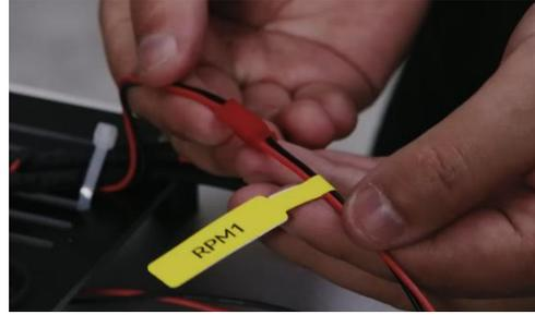
FIG 4-2-4 connected RPM line to RPM 1 port
