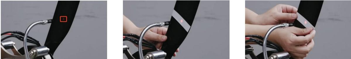
FIG 5-2-1 Stickers on the Propeller
