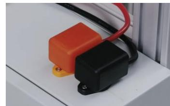
FIG 4-2-2 Power supply of ESC connected to current sensor output line
