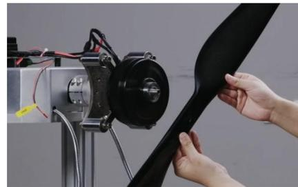
FIG 4-5-2 Check the motor rotate direction
