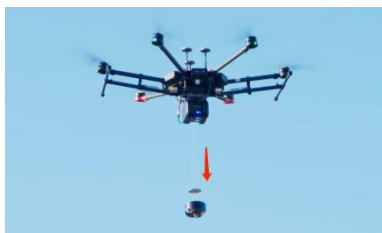
FIG 7-2-1 lower the rope to the ground
