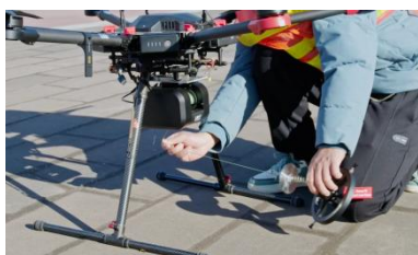
FIG 7-1-5 Lower the cable to a sufficient length
