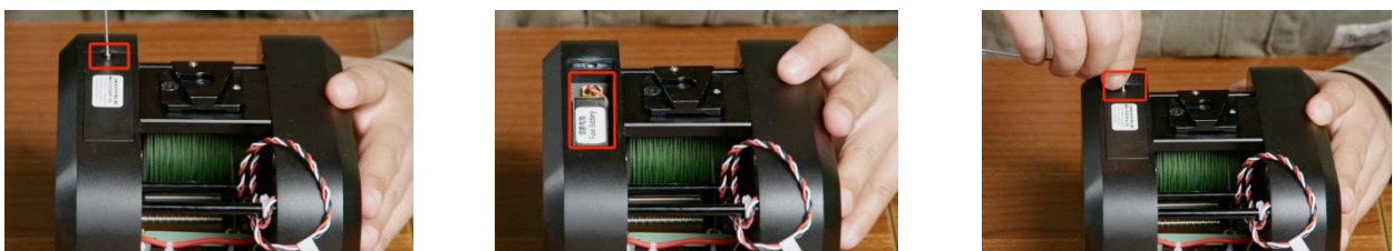
FIG 5-2-1 Fuse battery installation
