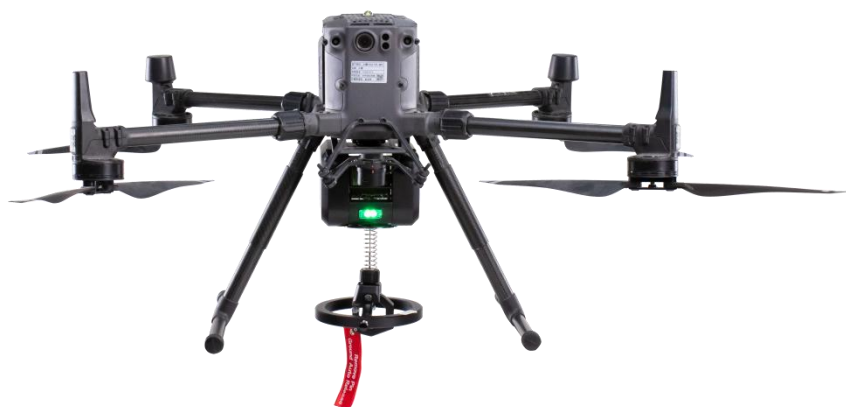
FIG 3-1-1 UAV platform equipped with XD-10 winch for drone system
