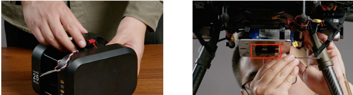
FIG 5-1-1 Show the quick-release mounting installation on drone
