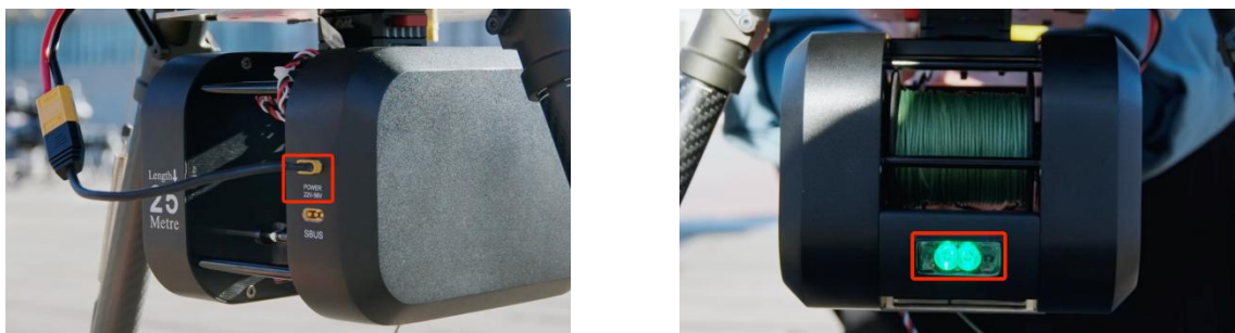
FIG 5-4-1SBUS Communication line connection
