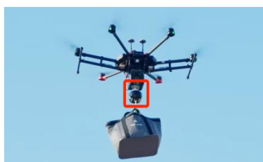
FIG 7-2-6 winch rises to the limiter
